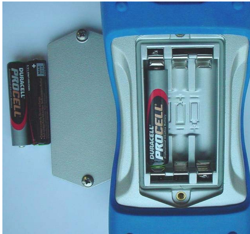
Figure 5: Replacement of batteries.
