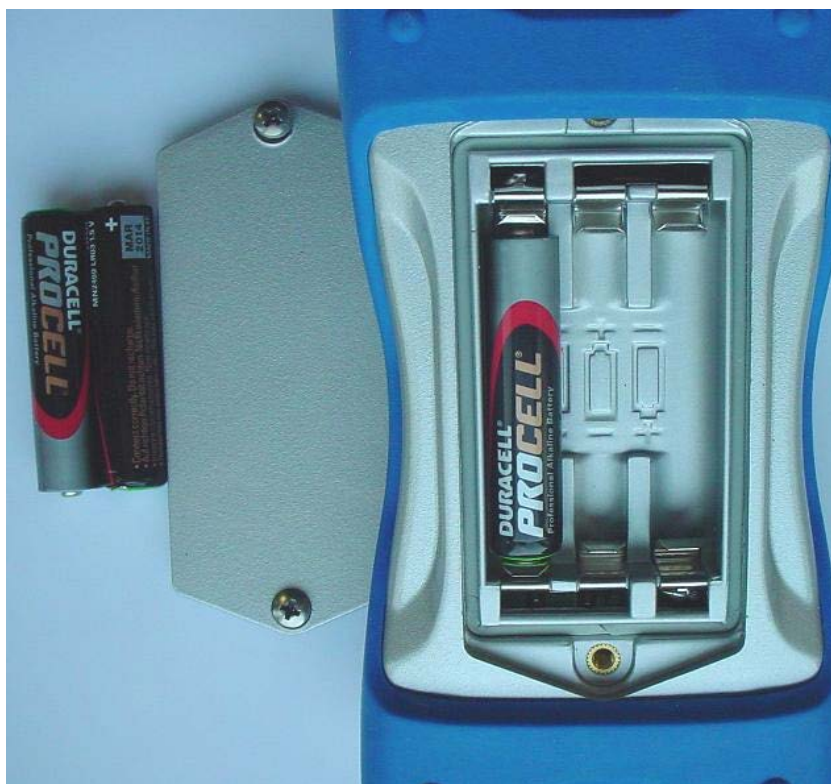
Figure 5: Replacement of batteries.
